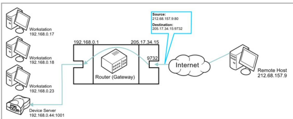
This shows the same set-up as above, but with a connection in progress. As you can see, the remote host can actually initiate a connection to the Device Server inside the network, because the router knows what to do with the data. Contrast the above diagram with the diagram on [How NAT Applies To Device Servers](#).
