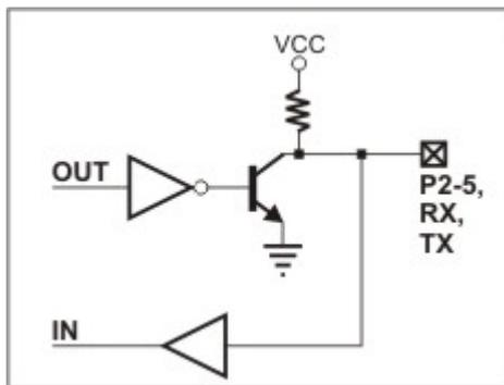
The serial-to-Ethernet firmware of the EM203 maps certain serial port functions onto the general-purpose I/O pins- these functions are shown in blue in the table above. For example, P5 is a universal input/output but the application firmware can be set to turn this line into the RTS output of the serial port. Therefore, depending on your application, you can view P5 as a general-purpose I/O line or specific control line of the serial port (RTS).
