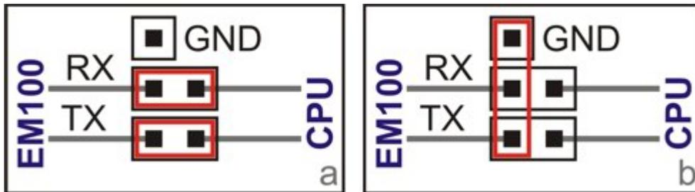
By providing the jumpers you are leaving a back-door access to the EM AND to the serial port of your main CPU. This may prove very useful during repairs, field service, etc. One final note: if you think that jumpers are too unreliable or you simply don't have enough space for them on the board then you can use solder jumpers instead.
