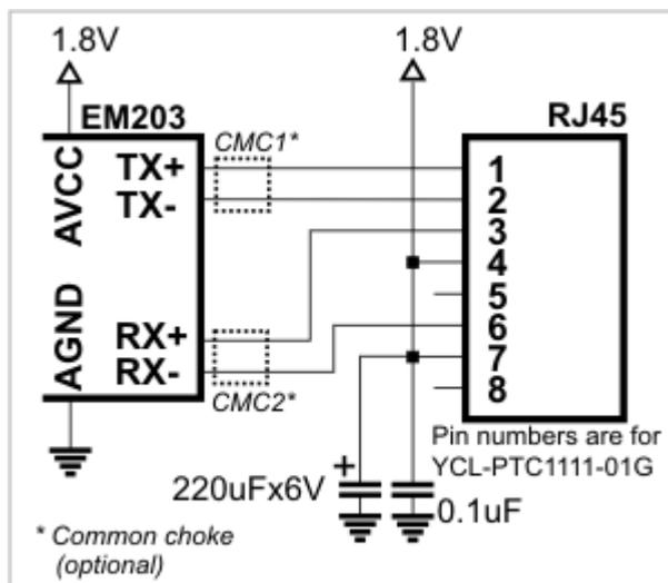
Ethernet port of the EM203 is of 10/100BaseT type. Onboard electronics of the EM203 do not include Ethernet magnetics, so magnetics circuitry must be connected externally to pins TX+, TX-, RX+, RX-, and AVCC. The AVCC pin outputs clean power for the magnetics circuitry, which is very sensitive to noise. The voltage on the AVCC output is 1.8V.
