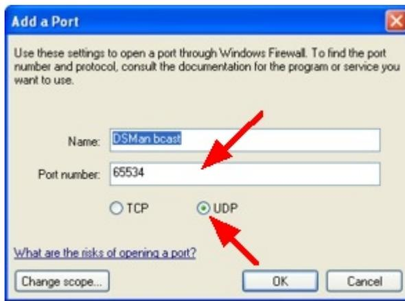
Input any meaningful name into the *Name textbox* (i.e. "DSMan bcast"- this is because what we are opening here is a port for *DS Manager's* auto-discovery broadcasts to work). In the *Port number textbox* input 65534- this is the port number that must be opened on your PC. Finally, select *UDP*- this is a protocol the *DS Manager* is using to find Device Servers on the network. Click OK when finished.
