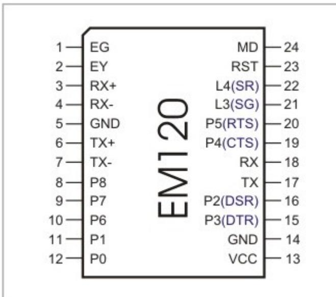
Click on the pin in the diagram above or one of the links provided below to learn more about EM120's I/O pins:
