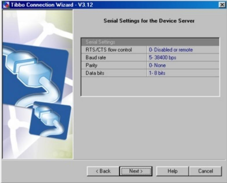
Unlike with the [VSP-to-DS link](#), the serial port parameters of the DS, involved in the application-to-DS link, cannot be adjusted via on-the-fly commands. You have to define fixed parameters that will be used by the DS at all times.
