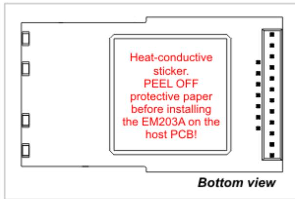
To further lower the operating temperature of the EM203A we advise you to arrange a copper area on the host PCB and in contact with the heat-conductive sticker. Best results are achieved when the copper area is larger, and also when two copper areas are provided on both sides of the host PCB and interconnected by a number of large vias.
