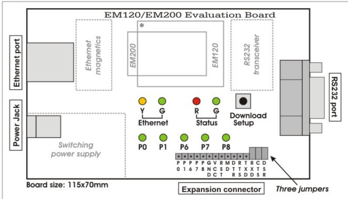
The EM120/200-EV Evaluation Board offers a convenient way of testing [EM120](#) and [EM200](#) Ethernet Modules. The board features the following components:
