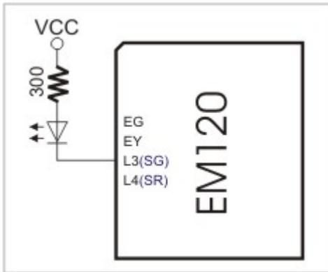
EG and EY lines reflect the status of the Ethernet port. The EG LED is normally ON, and is temporarily turned off whenever the EM120 receives a network packet. The EY is normally OFF, and is temporarily turned on whenever a data collision is detected on the Ethernet.
