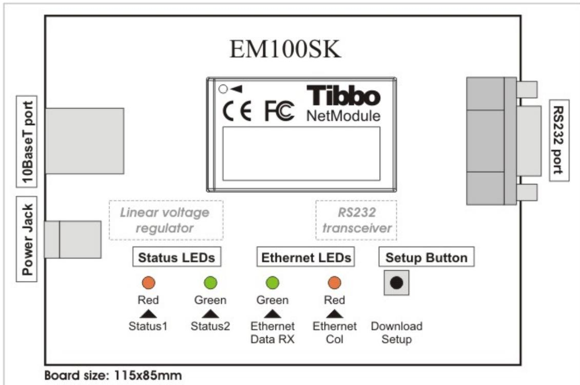
The EM100-EV Evaluation Board offers a convenient way of testing [EM100 Ethernet Module](#). The board features the following components:
