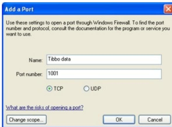
Notice, that you only need to open ports if your DS is going to connect to your PC. If it is the *VSP* (or application) on your PC that is going to connect to the DS then you don't need to setup the *Firewall*. This is because the *Firewall* doesn't block any connections that originate from within the PC.
