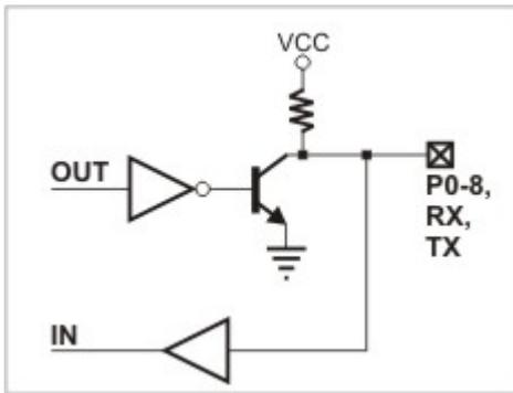
The [application firmware](#) of the EM120 maps certain serial port functions onto the general-purpose I/O pins- these functions are shown in blue in the table at the top of this topic. For example, P5 is a universal input/output but the application firmware can be set to turn this line into the RTS output of the serial port. Therefore, depending on your application you can view P5 as a general-purpose I/O line or specific control line of the serial port (RTS).
