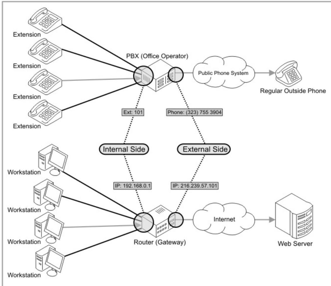
So, as can be seen above, a gateway has two addresses -- one on each network. And it can be very easily used for making an outbound connection. *But* -- what happens when you want to make an *inbound* connection?
