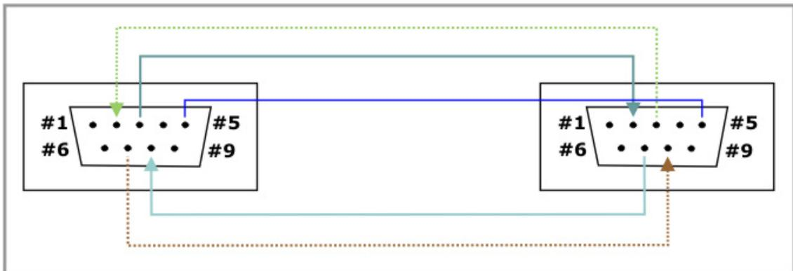
Like so. Both of the connectors for this cable should be "female". Tibbo makes exactly such a cable, called [WAS-P0005\(B\) DS-to-PC Serial Cable](#).
