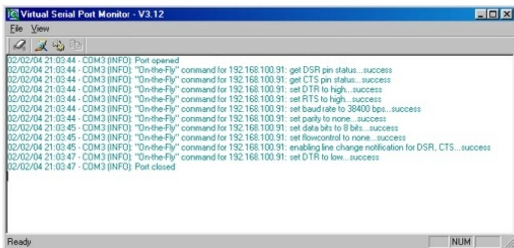
The *main window* displays the log of registered events. The simplest way to observe the work of the *Port Monitor* is to open the *VSP* from some application program and check what kind of data appears in the *Monitor* (sample output is shown on the screenshot above).
