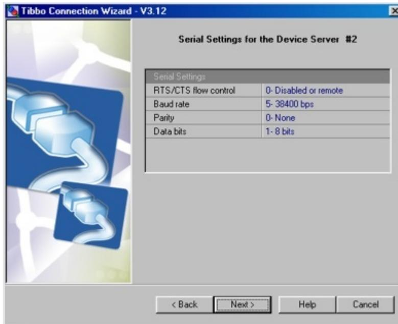
Unlike with the [VSP-to-DS link](#), the serial port parameters of the DS, involved in the DS-to-DS link, cannot be adjusted via on-the-fly commands. You have to define fixed parameters that will be used by this DS at all times.
