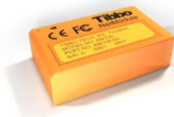
The EM100 is an Ethernet Module for onboard installation. Module hardware includes one 10BaseT Ethernet port (standard Ethernet magnetics are **integrated** into the Module), one serial port (CMOS-level) with a number of additional general-purpose I/O lines, and an internal processor, whose firmware acts as a bridge between the Ethernet and serial ports. Ethernet "side" of the Module connects directly to a standard RJ45 connector. Serial "side" interfaces directly to
