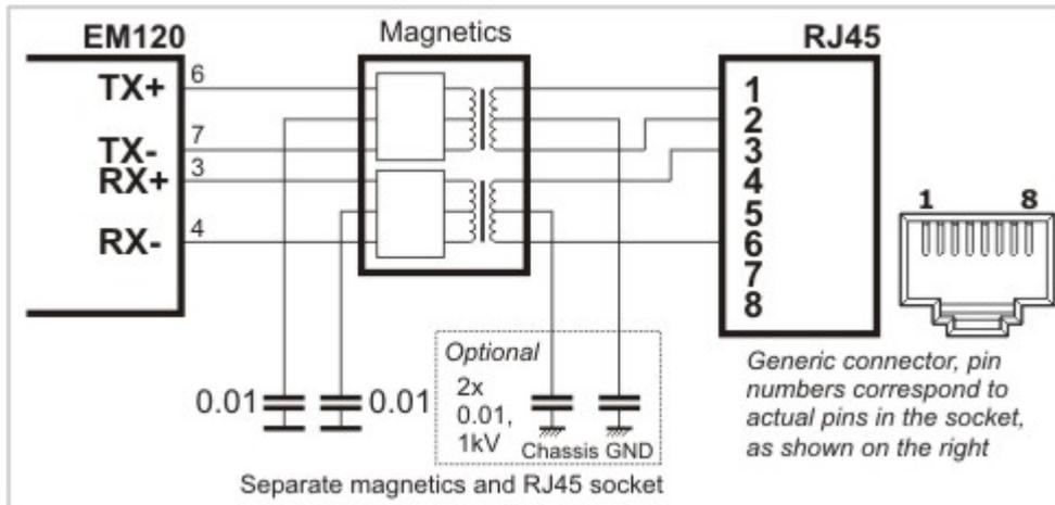
It is important to make the PCB wire connections between the Ethernet port pins of the EM120 and external magnetics circuitry as short as possible. Making the wires too long may cause the noise level generated by your PCB surpass the maximum radiated emission limits stipulated by FCC and CE regulations. Additionally, longer Ethernet lines on the PCB will make your board more susceptible to the damage from the ESD (electrostatic discharge).
