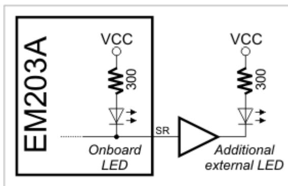
The firmware of the EM203A uses L3 and L4 as "status LEDs" which display various status information depending on what firmware is running at the moment.
