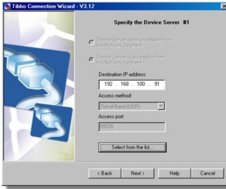
As [explained earlier](#), the DS #1 must be local, i.e. it must be located on the same network segment as the PC on which this *Wizard* is running (DS #2 can be local or remote). Because of that, the accessibility option is fixed at *Device Server is assessable from this network segment* (if the DS is local it is definitely must be accessible).
