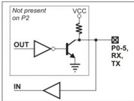
The [application firmware](#) of the EM100 maps certain serial port functions onto the general-purpose I/O pins- these functions are shown in blue in the table at the top of this topic. For example, P5 is a universal input/output but the application firmware can be set to turn this line into the RTS output of the serial port. Therefore, depending on your application you can view P5 as a general-purpose I/O line or specific control line of the serial port (RTS).
