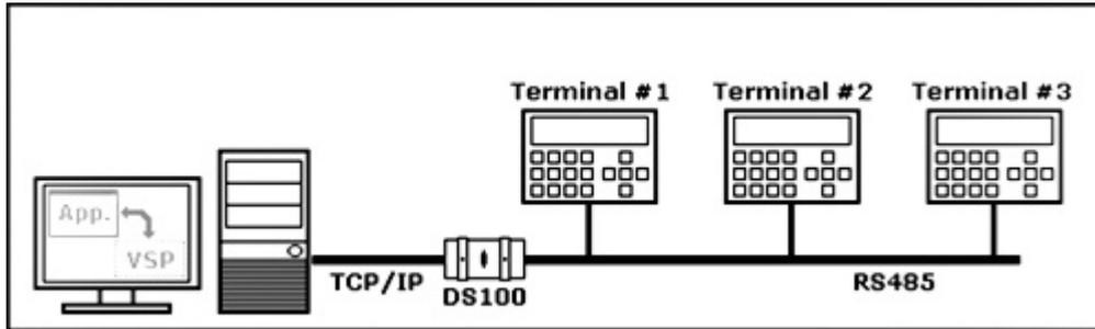
This will work, but only if the distance between the terminals is small. If the terminals are to be located far away from each other the RS485 network connecting them would have become very long thus defying the purpose of network-enabling this system! Much better solution would be to connect each terminal individually to its own DS (see figure below). This way there would be no RS485 network whatsoever.
