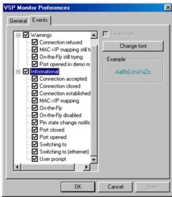
When the *Monitor* is installed all events are enabled and three different font types are selected for the informational, warning, and error events:
