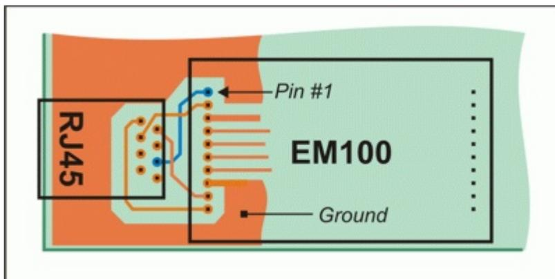
Another important point. Do not create a ground plane in the vicinity of the RJ45 connector and RX-, RX+, TX-, and TX+ lines. The ground plane should "wrap around" the RJ45 area, but not cross any of the 4 interface wires. This is very important! Providing a ground plane beneath the connector area will make your device very susceptible to the ESD.
