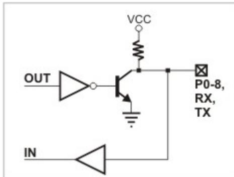
[Device server application firmware](#) of the EM1000 maps certain serial port functions onto the general-purpose I/O pins- these functions are shown in blue in the table at the top of this topic. For example, P5 is a universal input/output but the application firmware can be set to turn this line into the RTS output of the serial port. Therefore, depending on your application you can view P5 as a general-purpose I/O line or specific control line of the serial port (RTS).
