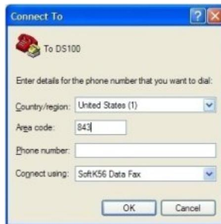
By default, HyperTerminal tries to configure a connection using a modem (if one is installed). However, we don't need a modem for our configuration. As covered above, we usually need one of two connection types: TCP/IP connection, or a direct serial connection.
