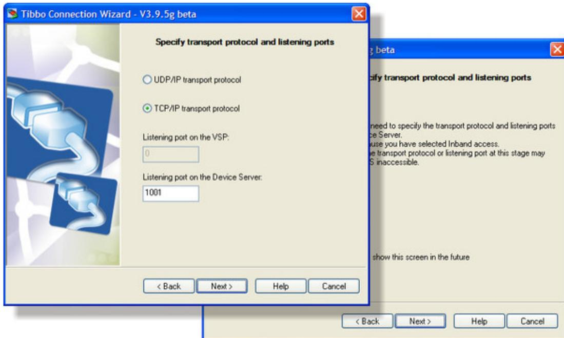
In general, we recommend you to stick to the TCP/IP, unless the application requires that the UDP/IP protocol is used. Since the *Wizard* can only setup the transport protocol on the DS side of this connection, it is your responsibility to setup the application side accordingly.
