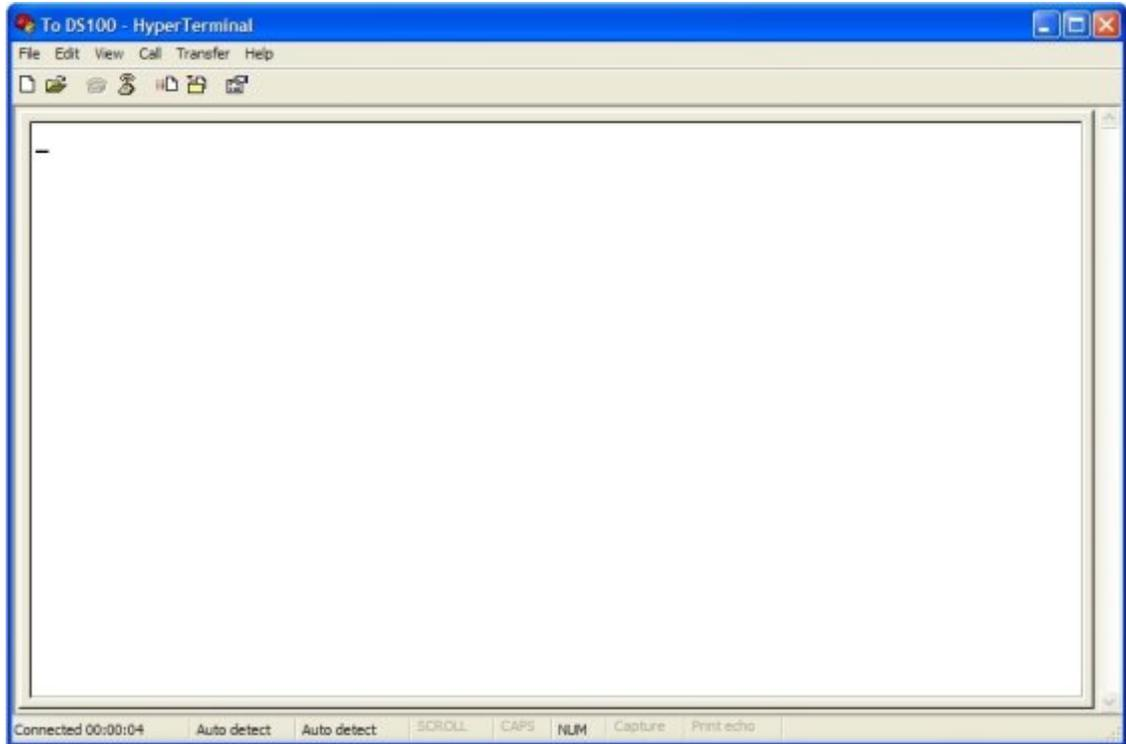
Basically, HyperTerminal lets you type characters (or send files in specific protocols) from your computer, which is acting as a TERMINAL (computer originating or receiving communications), to another computer or device (such as a DS100) which is connected to it.
