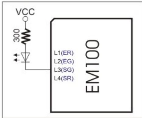
The firmware of the EM100 assigns specific functions to these LED control lines—these functions are shown in blue in the table at the top of this topic.
