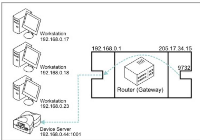
As you can see, this is a *static* configuration. **This is configured on the router itself -- it is not related to any Tibbo equipment.** The diagram above shows the setup itself -- no connection is in progress, but the router knows what to do when it gets data to port 9732.
