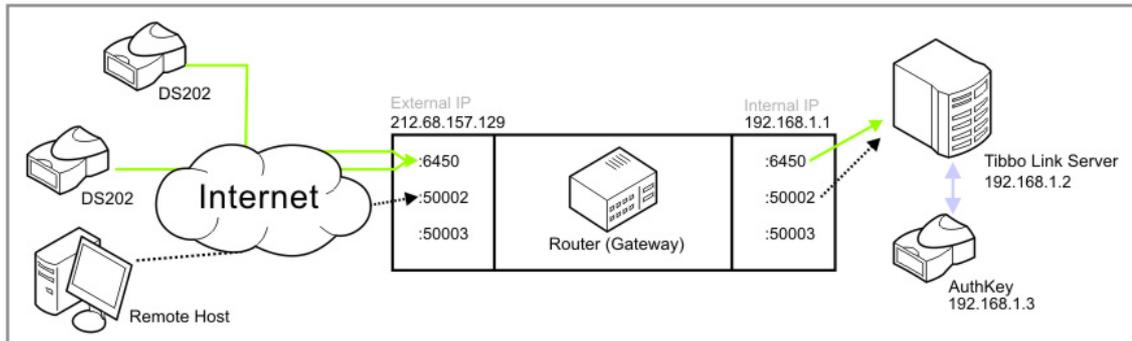
The Device Servers connect to port 6450, which is the default LinkServer login port for Device Servers. The remote host connects to port 50002, which is one of the ports assigned to Device Servers within the LinkServer, so it actually reaches a Device Server through this connection (via the LinkServer).
