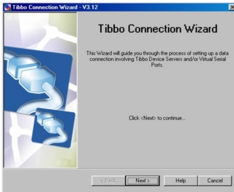
*Connection Wizard* offers a selection of jobs that help you setup several kinds of typical data links involving Tibbo Device Servers and *Virtual Serial Ports (VSPs)*. For example, a [VSP-to-DS](#) job helps you create a *VSP* on the PC, and then configure this *VSP* and the Device Server (DS) of your choice to work with each other.
