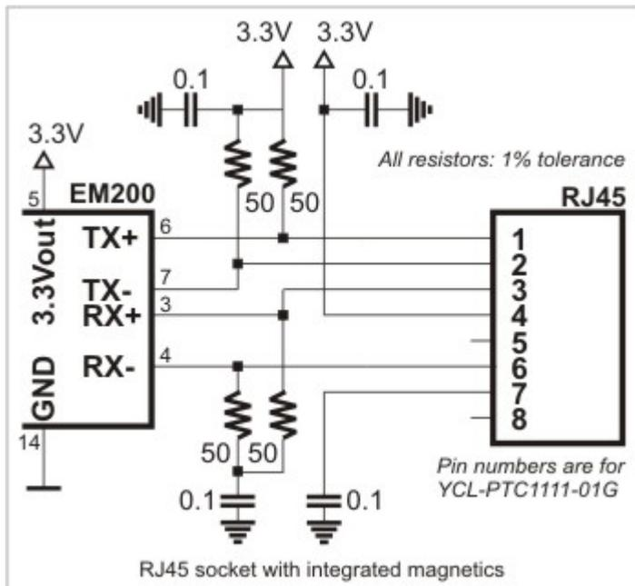
It is important to make the PCB wire connections between the Ethernet port pins of the EM200 and external magnetics circuitry as short as possible. Making the wires too long may cause the noise level generated by your PCB surpass the maximum radiated emission limits stipulated by FCC and CE regulations. Additionally, longer Ethernet lines on the PCB will make your board more susceptible to the damage from the ESD (electrostatic discharge).
