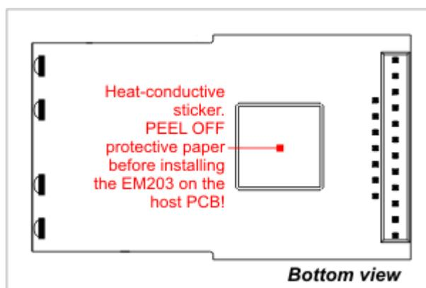
To further lower the operating temperature of the EM203 we advise you to arrange a copper area on the host PCB and in contact with the heat-conductive sticker. Best results are achieved when the copper area is larger, and also when two copper areas are provided on both sides of the host PCB and interconnected by a number of large vias.
