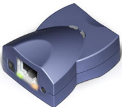
The DS203 is a Serial Device Server for external use. Device hardware includes one Auto-MDIX\* 10/100BaseT Ethernet port, one RS232 serial port and an internal processor that "glues" network and serial sides together.
