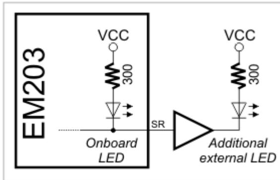
The firmware of the EM203 uses L3 and L4 as "status LEDs" which display various status information depending on what firmware is running at the moment.
