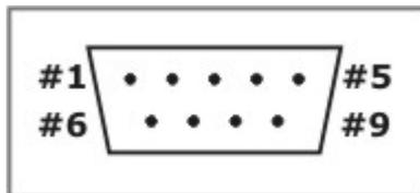
The serial port connector of the DS100 is of DB9M type. The DS100 is supplied in two models: the DS100R with RS232 port and DS100B with universal RS232/RS422/RS485 serial port. Notice, that there are no terminators (usually required at the ends of RS422 and RS485 buses) inside the DS100B. Termination circuits are present on the [TB100 Terminal Block Adaptor](#) that can be optionally supplied with the DS100B.
