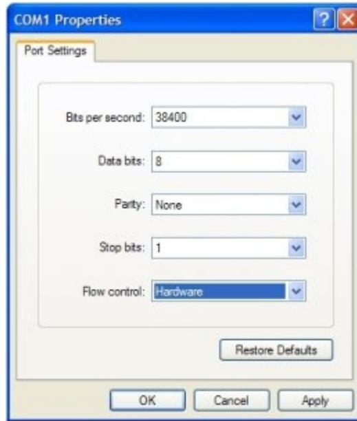
2) **If you would like to simply communicate using the DS**, the correct settings are those which were configured using the *DS Manager* or *Connection Wizard* for this DS. They can be 38400, 8, N, 1 but they can also be different.
