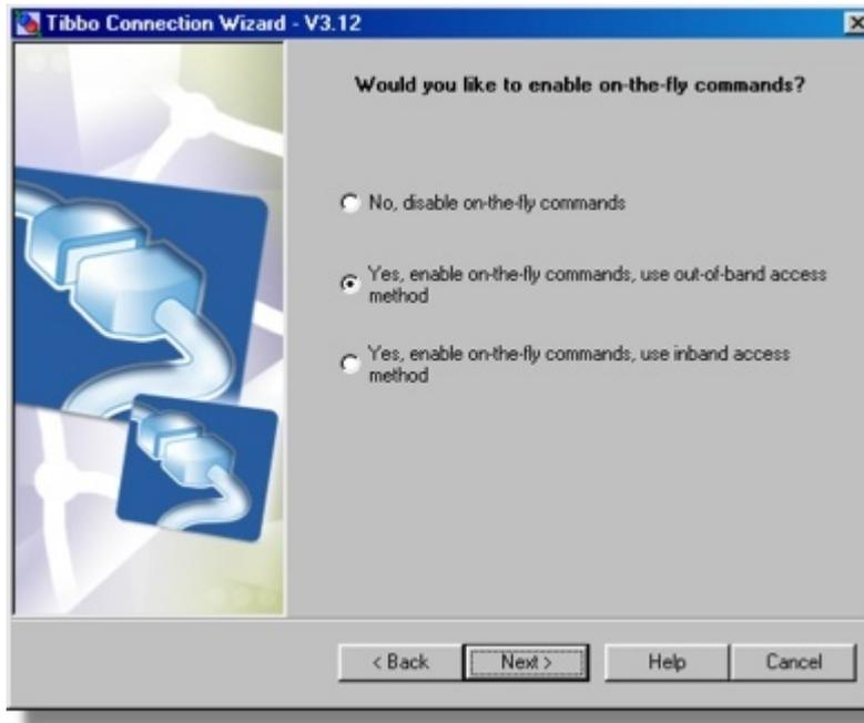
The VSP-to-DS connection can be arranged in such a way that the serial port of the DS is always setup as required by the "serial" application. For example, if the application that opens the *VSP* selects the baudrate of 9600 bps, then the baudrate of the DS serial port is immediately set to this baudrate as well.
