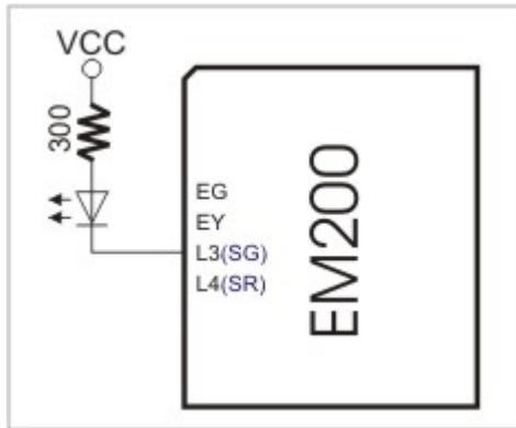
EG and EY lines reflect the status of the Ethernet port. The EG LED is switched on whenever a live Ethernet connection is detected by the EM200's Ethernet port. The EG LED is momentarily switched off whenever the EM200 receives a network packet. The EY shows whether current Ethernet link is of 10BaseT type (EY off) or 100BaseT (EY on).
