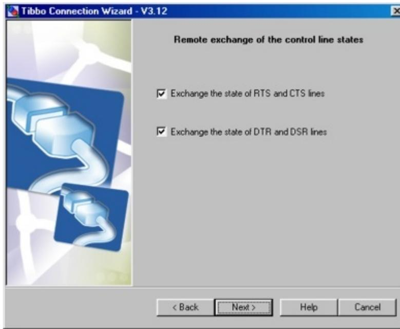
When this feature is enabled, a change in the state of the CTS (DSR) input on one DS causes a corresponding change on the RTS (DTR) output of the other DS. In effect, this achieves complete emulation of the serial cable over the network: not only the serial data is seamlessly transmitted between the serial ports of two Device Servers, but also the control lines appear to be interconnected.
