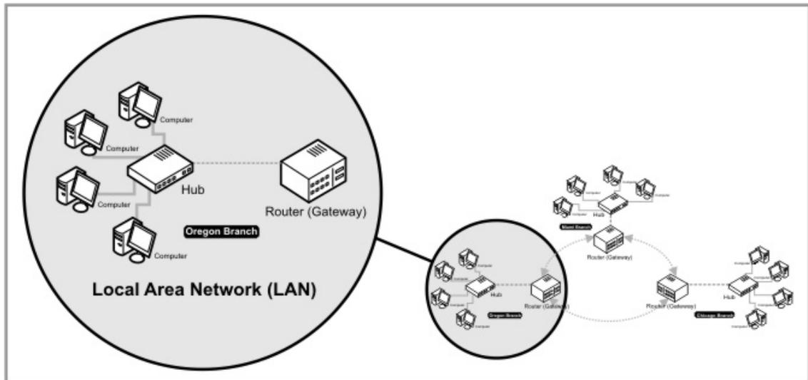
There are certain types of communication which are unique to a LAN. One such type is called 'broadcast' communication. This is where one node (station, host, computer) on the LAN 'shouts out' so that all other nodes hear the message. This is similar to pressing the 'announcement' button on an office telephone, and using all the phones connected to the system to broadcast a message to all employees (through the speaker of the phone).
