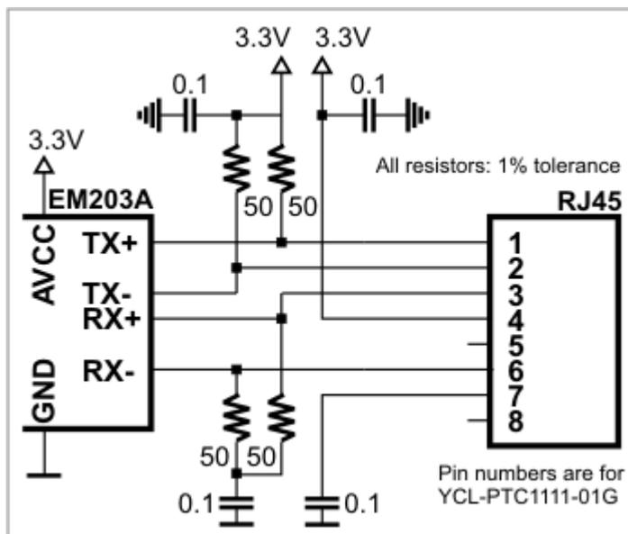
Ethernet port of the EM203A is of 100/10BaseT type. Onboard electronics of the EM203A do not include Ethernet magnetics, so magnetics circuitry must be connected externally to pins TX+, TX-, RX+, RX-, and AVCC. The AVCC pin outputs clean power for the magnetics circuitry, which is very sensitive to noise. The voltage on the AVCC output is 3.3V.
