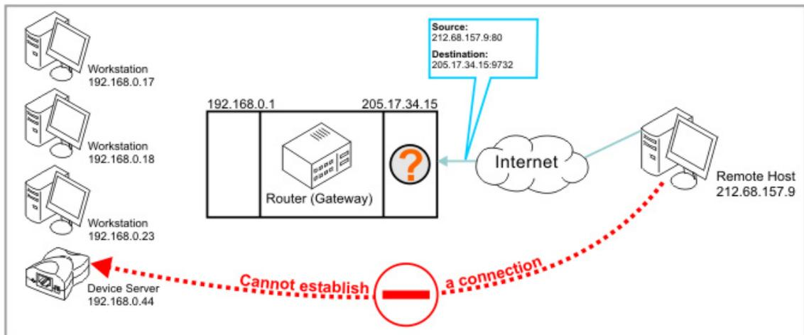
As can be seen above, when you have a DS in a LAN, behind a NAT router, you cannot simply establish a connection from outside. The port isn't mapped anywhere, so the router drops the packet.
