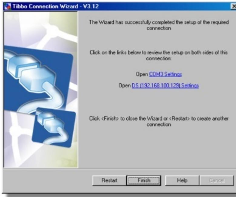
For example, if you've just finished the [VSP-to-DS](#) job then you will see two links as shown on the screenshot above. The first one opens the [VSP properties dialog](#), the second one- [DS settings dialog](#). This provides a comfortable way of reviewing the setup and making changes (if necessary) right from inside the *Wizard*.
