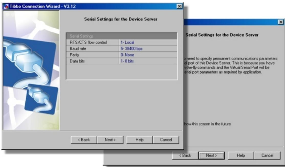
Values entered on this screen are saved into the [serial settings](#) of the DS. Once set, they remain unchanged even after the DS is switched off. The serial port of the DS will always use these values unless temporary overriding parameters are received from the *VSP* (in the form of the on-the-fly commands- if you have enabled them on the [previous step](#)).
