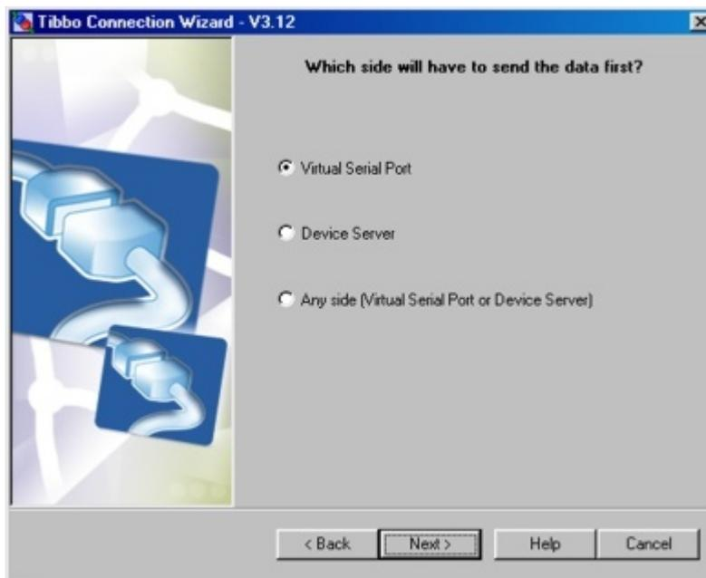
Notice, that asking "who will be the first to send the data?" is not the same as asking "which side will be establishing the data connection to the other side?"\* When making your choice imagine that there is no network at all and the serial device is attached to the COM port of the PC directly. Now, which side sends the
