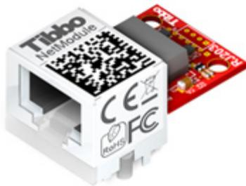
The RJ203 is an "Ethernet front-end" module that contains 10/100BaseT Ethernet magnetics and a standard RJ45 jack. Module's magnetics are designed to work with Davicom's DM9000A Ethernet controller.
