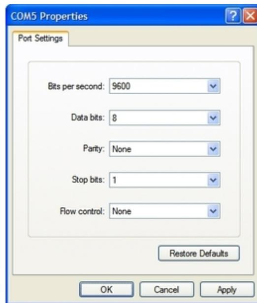
After setting the desired parameters, click OK. That's it! You've now established a connection with the DS100 via the *Virtual Serial Port*. Continue on to [Using HyperTerminal to Test a Connection](#).
