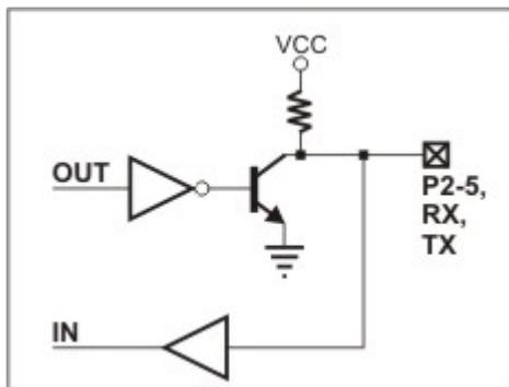
The serial-to-Ethernet firmware of the EM203A maps certain serial port functions onto the general-purpose I/O pins- these functions are shown in blue in the table above. For example, P5 is a universal input/output but the application firmware can be set to turn this line into the RTS output of the serial port. Therefore, depending on your application, you can view P5 as a general-purpose I/O line or specific control line of the serial port (RTS).
