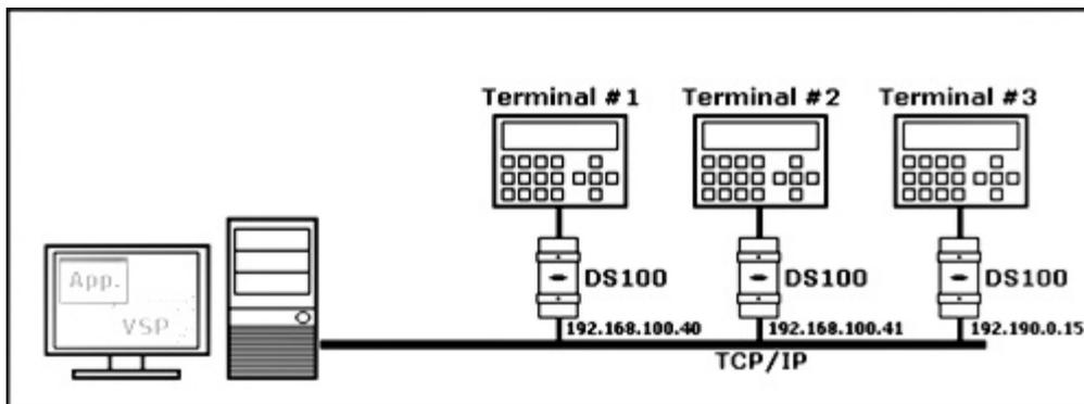
The problem here is that each DS (and hence, each terminal) will now have its own IP-address and this means that a single *VSP* will have to switch between these IPs as needed (remember that on the original RS485 system the application software communicated with all terminals on the RS485 bus through a single COM port!).
